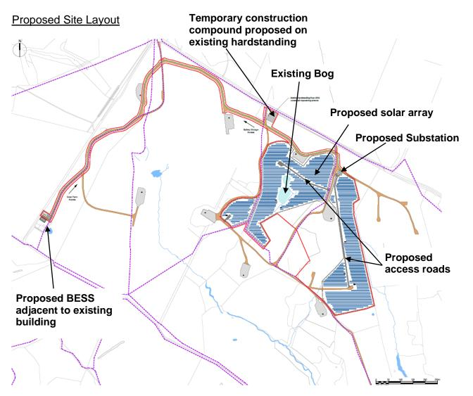
The ground area for the installation of PV panels has been reduced since the application was submitted from a coverage of approximately 22.6ha to 14.1ha which is in order to address ecology issues. Due to advances in solar equipment it is still expected to produce the same amount of energy and would be sufficient to offset the annual electricity usage of approximately 2,500 homes in Burnley.
